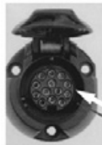
Fig. 3 - Socket body (containing female socket terminals) fitted to the car
