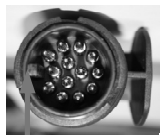
Incorrect alignment Fig. 7
