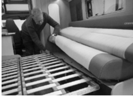
Step 6: Lowering the bed frame, ensure hooks locate into the off side bed base top
