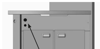
Typical 2nd thermostat and switch arrangement
