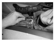
Pull the turning handle of the locking mechanism upwards
