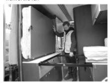
• Secure the front support rail in position using the magnets with the handle facing upwards
