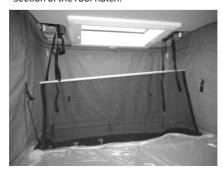
Fall-Out protection is provided when using the upper bunk. The net is stored under the mattress and is secured to the handles on the roof using the adjustable straps on the upper rail.
