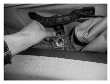
Turn the locking handle in a counter clockwise direction to release
