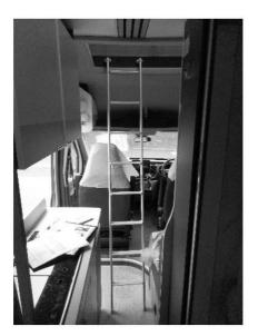
To access the upper bunk use the folding bunk ladder stored in the rear nearside bed. The ladder hooks on to the brackets on the front section of the roof hatch.
