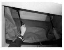
Pull the roof down carefully using the strap at each side together ensuring the tent fabric will not be jammed in this process.
