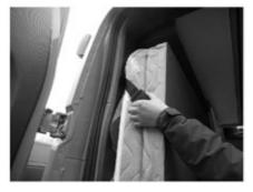
Release the strap securing the nearside bed and hold the bed as you back away towards the front of the van
