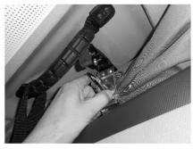
Pull the turning handle downwards and turn it in a clockwise direction to tighten the locking mechanism.
