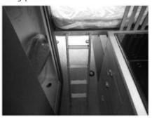
• Attach the short bunk ladder to the brackets on the front of the bed base
