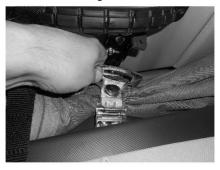
Release the locking mechanism from the magnet and hook on to the bracket on the frame
