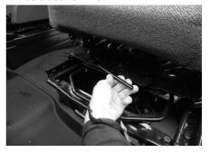
To turn the swivel, slide the BLACK lever forwards and adjust to the required angle. Before driving off ensure the locking mechanism is fully secure.
