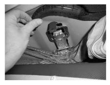
Unhook the locking mechanism from the bracket and fold up and fix on the magnet on the roof
