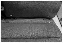
Top tether anchor points are fitted on the upper seatbelt stanchion and are accessed by removing an insert on the backrest cushion.
