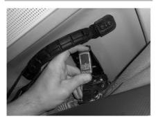
Close the Click-Lock of the roof (driver's side as well as passenger's side) to ensure the locking mechanism cannot pull free.
