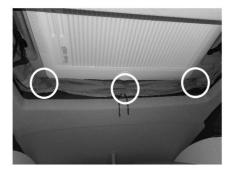
Fold up the remaining tent fabric thoroughly in the front area and fix using the three Velcro fasteners
